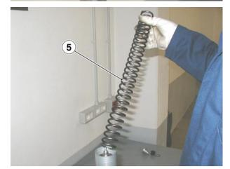
• Fit aluminium shim and plastic bushing (4) onto spring (5).
