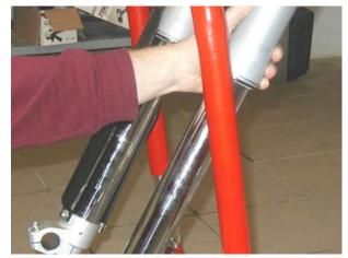
Support the fork leg and tighten the two screws on top and bottom plate.
