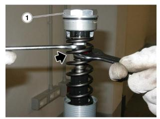
Tighten the cap (1) onto sleeve (3).
