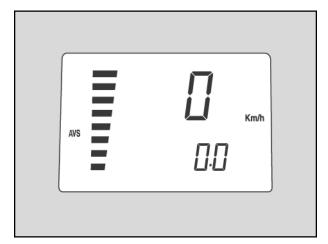
To reset TRIP and corresponding AVERAGE SPEED (AVS) counter press MODE or SCROLL for more than five seconds, with vehicle stopped, and value displayed in area B of the display will change into four dashes. Dashes will turn into four zeroes when button is released (000.0).
