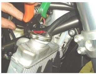
Working on the right side, loosen the lower screw and collect the nut and washer on the left side.
