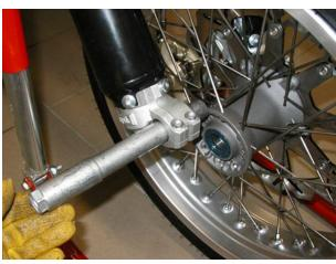
Working on the left side, partially tighten the front wheel shaft nut.
