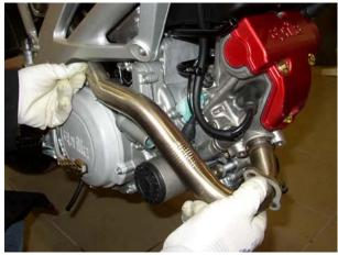
Loosen and remove the two screws from rear cylinder exhaust manifold.
