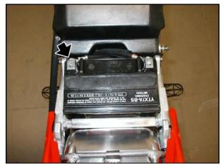
Loosen and remove the positive cable screw, keep the fastener.
