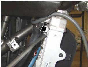
• Slide out the radiators in a downward motion.
