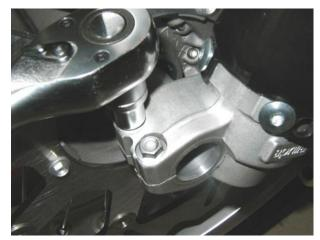
• Working on the right side, slide out the wheel shaft.
