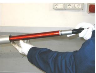
Slide out the dust seal (1) from the sleeve prising it out with a screwdriver.
