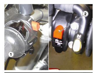
• Turn the key and set the ignition switch to position "O".
