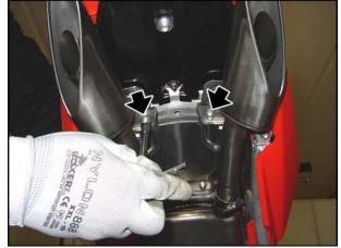
• Working on either side, remove the mounting spring.
