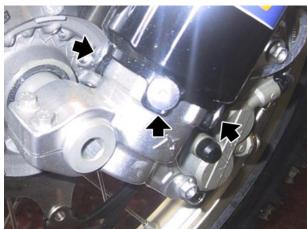
Support the fork leg and loosen the screws from top and bottom plate.
