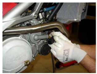
• Working on either side, release the clamps.
