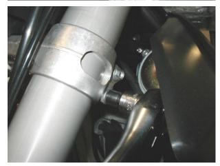
Install the leg guard, position and tighten the three screws.
