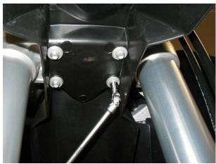
• Tighten the two mudguard front screws.
