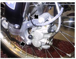
Working on the left side, loosen and remove the front wheel shaft nut.
