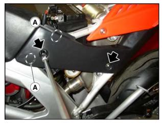
Unscrew and remove the tank retaining screw and collect the pilot bush.
