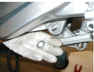
Slide out the swinging arm/levers shaft.
