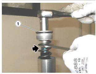
• Tighten the cap (1) onto sleeve (3).
