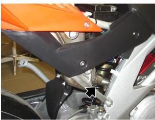
• Working on either side, loosen and remove the two screws, collect the washers.
