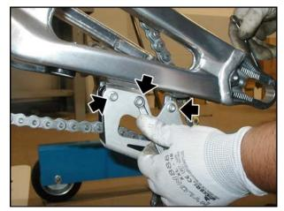
• Move the chain to the side completed with chain guide.
