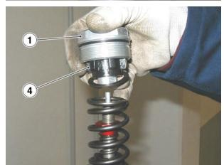
• Remove the spring (5). Let oil drip from the spring into the sleeve to avoid topping up or fluid change.
