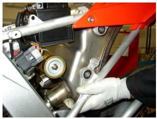
Loosen and remove the two screws from front cylinder exhaust manifold.
