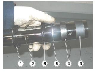
Bushing (3) and guide ring (4) can be removed using a small screwdriver; then the following parts can also be removed:
