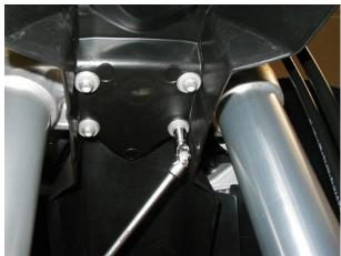
• Tighten the two mudguard front screws.
