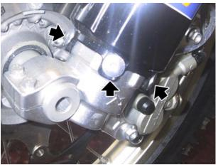
• Fit the speed sensor and tighten the two screws.
