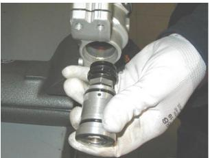
• Slide out the complete damper rod.
