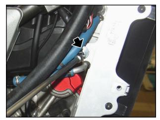
Working on the right side, loosen the upper screw and collect the nut and washer on the left side.
