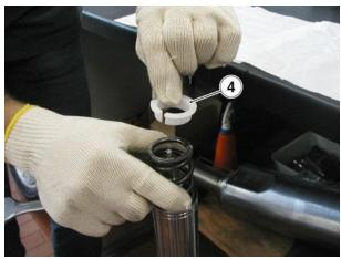
Remove the spring (5). Let oil drip from the spring into the sleeve to avoid topping up or fluid change.
