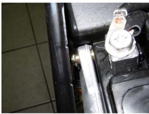
Remove the tank retaining pin from the side without lower side body panel.
