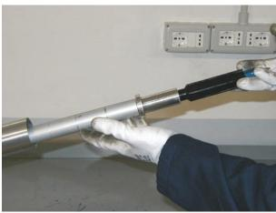
Fit and tighten the bottom plug.
