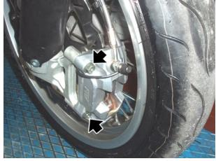
Working on the left side, loosen and remove the front wheel shaft nut.
