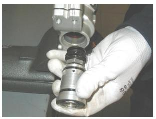
Slide out the complete damper rod.
