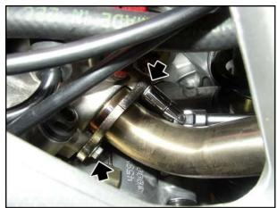
• Remove the rear cylinder exhaust manifold.
