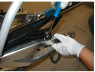
Loosen and remove the three screws from chain guide and collect the two nuts.
