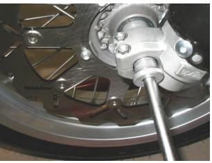
Working on either side, loosen the wheel shaft pinch holts
