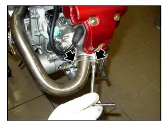
• Remove the front cylinder exhaust manifold and collect the clamp.
