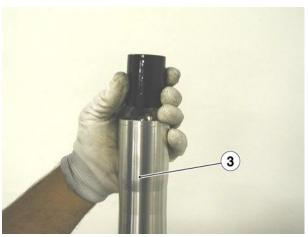
Pour fork fluid inside the sleeve (3) up to the correct level that can be measured by inserting a graduated rod inside sleeve (3).
