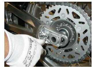
Using a rubber mallet, slide out the wheel shaft on the left side of the vehicle, collect the shims and remove the wheel from the rear end.
