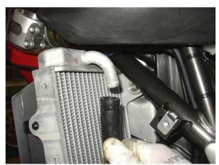
Working on the left side, release the clamp and disconnect the hose.
