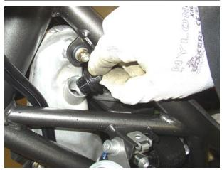
Remove the oil tank from below.
