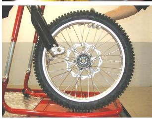
• Working on the right side, fit the wheel shaft.
