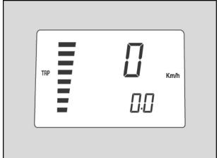
Press again MODE, if vehicle is stopped, or SCROLL, if vehicle is running, and TRIP indication will switch to AVERAGE SPEED (AVS) indication, as calculated within the trin
