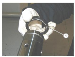
Fit the complete damper rod fully home in the fork leg.
