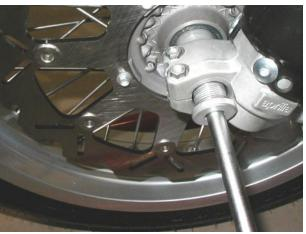
Working on either side, loosen the wheel shaft pinch bolts.
