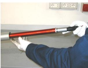
Fit and tighten the bottom plug.
