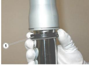
Remove the snap ring (2) from inside the sleeve, using a screwdriver.
