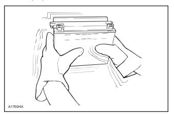
5. Readjust the electrolyte level to the UPPER LEVEL line.
