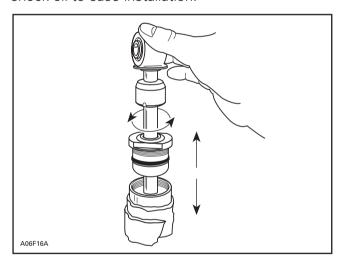
Seal carrier should be installed close to piston assembly. Careful inspection of damper oil capacity is required to insure that no air is in damper body during assembly.
