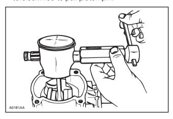
NOTE: The PTO cylinder or fan housing have to be removed to give access to MAG piston pin with the puller.
