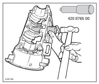
NOTE: Bearing shielded side must be facing rotary valve.
