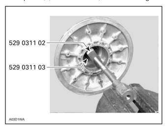
Mount puller screw head in a vise.
