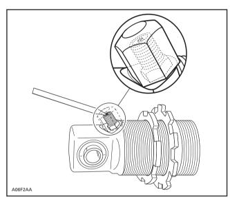
Use tools (P/N 861 7439 00) to remove damper spring by unthreading spring pre-load rings, then removing spring retainer.
