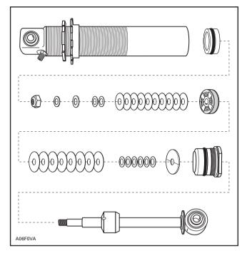
NOTE: As a general rule we suggest replacing the damper rod lock-nut after 4 rebuilds to ensure good locking friction.
