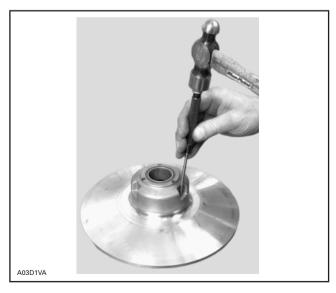
Install support plate (P/N 529 0311 03) inside sliding half.
