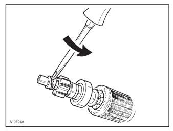
Twist screwdriver to separate stop collars no. 12 thus giving access to circlip no. 13.
