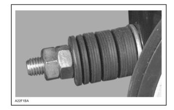
Tighten nut 3/4 turn after contacting washers for better deep snow performance. Maximum preload is 3 turns after nut touching washers. This last adjustment is for trail riding with or without a load and for pulling a load.
