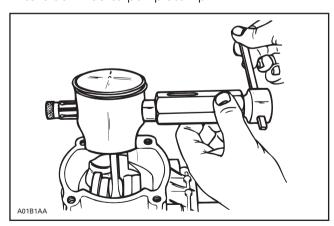
NOTE: 0.25 mm oversize piston and rings are available if necessary except for 454 engine.
