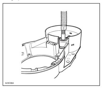
Support fan housing no. 12 with a ring. With a punch, working all around bearing no. 10 inner race, drive bearing out of fan housing. Keep shims for installation.
