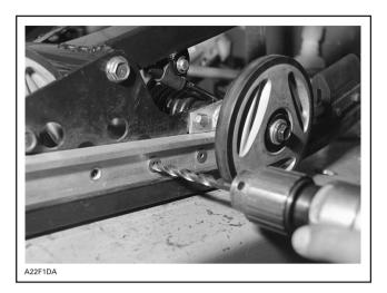
Rivets can be substitued by M8 x 20 bolts and nuts.
