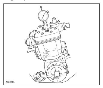
Interval between cylinders must be exactly 180°. Any other reading indicates a misaligned (twisted) crankshaft.
