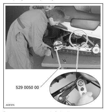
Remove nut on top end of shock.
