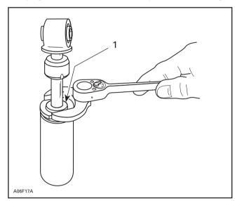
1. Torque seal carrier to 88-98 N•m (64-72 lbf•ft)
