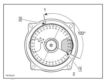
Step 1: Align 360° line of degree wheel here Step 2: Find 132° on degree wheel and mark here
