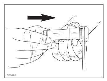
Mount piston over connecting rod with the letters "AUS" (over an arrow on the piston dome) facing in the direction of exhaust port.
