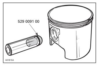
NOTE: The circlip on the opposite side can be installed before pin installation, the tool will easily go out.
