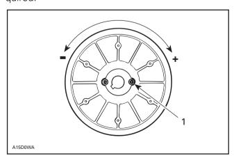
1. Allen screw with jam nut
