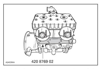
Apply Loctite 242 (P/N 413 7030 00) on cylinder screw threads.
