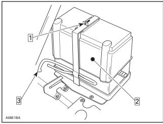
Step 1 : Unfasten and open Step 2 : Lift protective boot Step 3 : Remove vent tube
