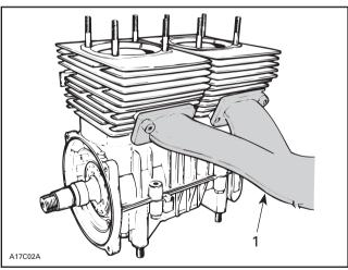
1. Or use exhaust manifold to align cylinders
