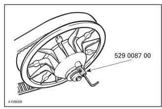
Restrain Allen screws with the wrench and tighten nut with the socket using socket handle provided in tool box.
