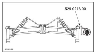
TYPICAL — DSA CAMBER ADJUSTMENT SET-UP
