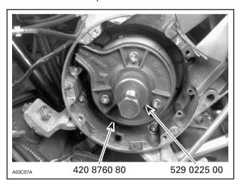
To remove magneto flywheel retaining nut no. 3, install puller ring (P/N 420 8760 80) and M8 x 20 screws.
