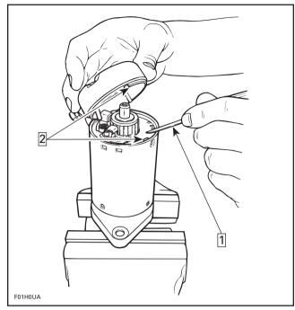
Step 1 : Retaining brush holder with a screwdriver
