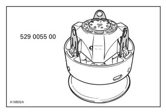
Make sure to align governor cup arrow with sliding half and fixed half mark.
