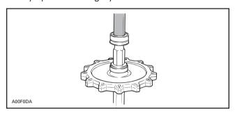
The bearing on the splined side of axle must be pushed until it is seated on shaft shoulder. The end bearing housing bearing must be flush with end of drive axle. Each bearing must have its shield facing the sprocket.
