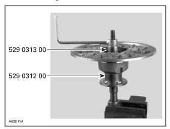
**IMPORTANT:** Large bushing retaining screws and washers must be removed before small bushing installation.
