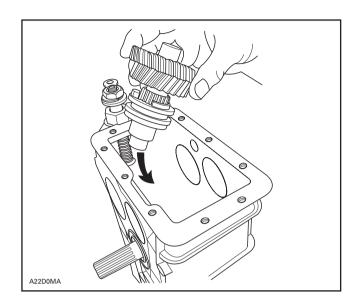
Install shim and bearing on LH side.
