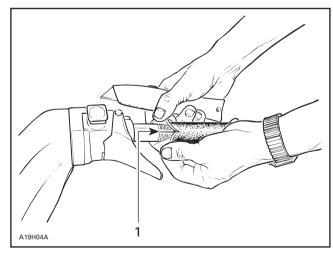
1. Gap in the heating element opposite the wires
