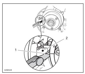
ADJUSTING TRIGGER COIL AIR-GAP
