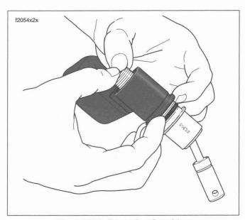
Figure 2-58. Removing Cartridge
