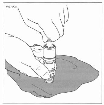
Figure 2-59. Compress Spring and Retaining Ring
