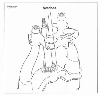
Figure 2-107. Pry Points: FLSTSC
