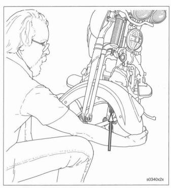
Figure 2-126. FLSTSC Front Fender Bracket
