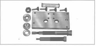
Part No. HD-42325-A Camshaft Needle Bearing Remover/Installer
