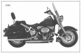
Figure 4-30. Oxygen Sensors (Inboard Side Of Exhaust Pipes)
