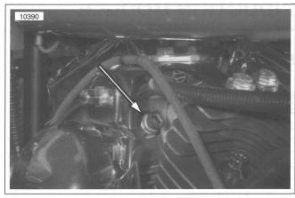
Figure 4-19. Engine Temperature Sensor
