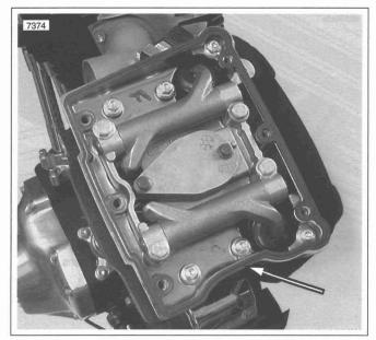
Figure 3-47. Rocker Cover Gasket Indent (Front Cylinder Shown)
