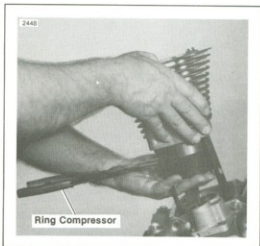
Figure 3-24. Slipping Cylinder Over Piston
