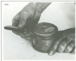
Figure 3-20. Measuring Ring Side Clearance
