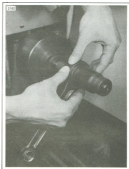
Figure 3-50. Lapping Connecting Rod Bearing Races
