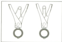
Figure 3-26. Hose Clamp Connection
