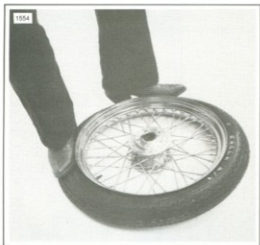
Figure 2-32. Loosening Tire Beads
