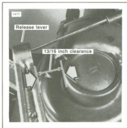
Figure 6-30. Release Lever Measurement
