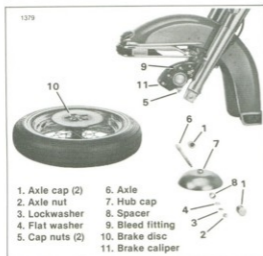
Figure 2-1. FL Front Wheel Mounting — 1978½-1980
