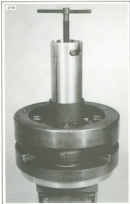
Figure 3-48. Pulling Bearing from Sprocket Shaft
