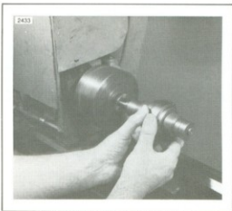
Figure 3-46. Lapping Connecting Rod
