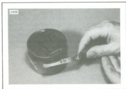
Figure 3-22. Measuring Ring Side Clearance
