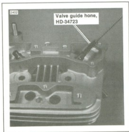
Figure 3-9. Honing Valve Guides
