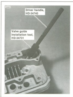
Figure 3-10. Installing Shoulder-less Valve Guides
