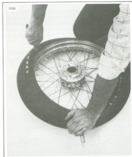
Figure 2-37. Starting Second Bead on Rim
