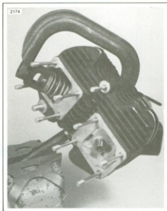
Figure 3-4. Compressing Valve Spring
