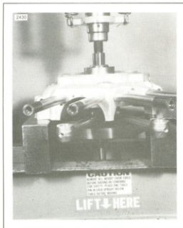
Figure 3-39. Pressing Flywheels Out of Crankcase
