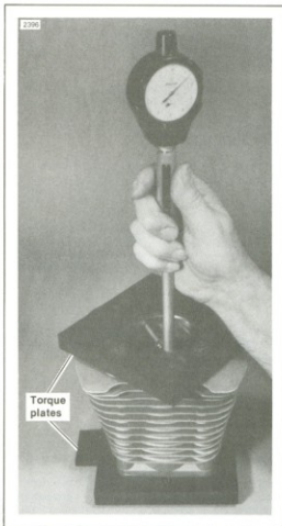
Figure 3-19. Measuring Cylinder Bore
