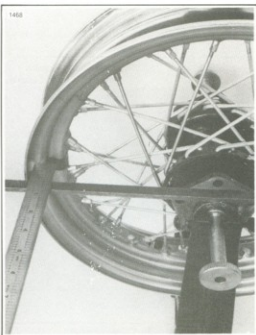
Figure 2-27. Centering 16 in. and 21 in. Hub
