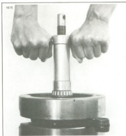
Figure 3-58. Pressing Bearing on Sprocket Shaft
