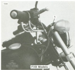
Figure 2-87. Throttle Cable Routing — 1981
