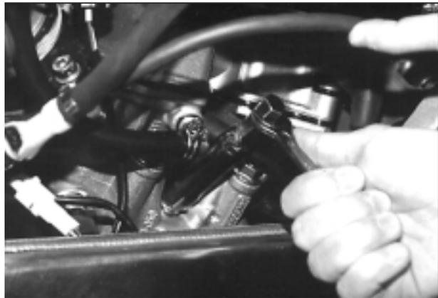
To remove and clean the spark plug, proceed as follows:
